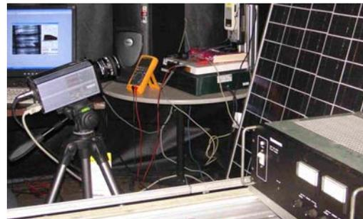
**Figure 9:** Electroluminescence Crack Detection (ELCD)
