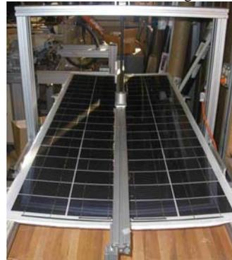
**Figure 14:** Laminate flex tester
