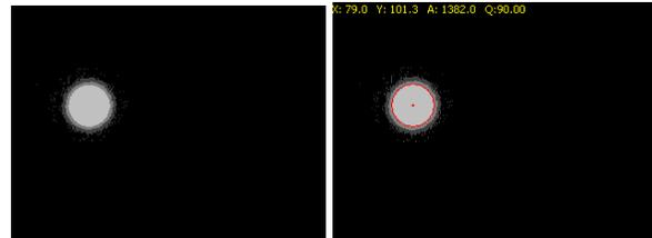
Fig. 2. Image of the sun acquired using pinhole setup, before and after circle-finding.
