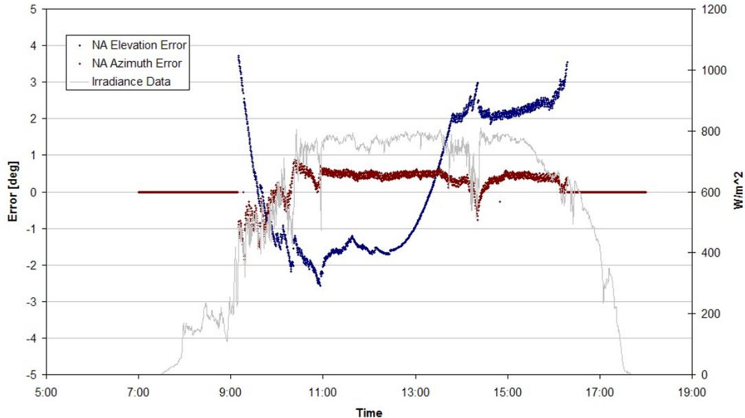
Fig. 6. Tracker performance as measured on a cloudy day.
