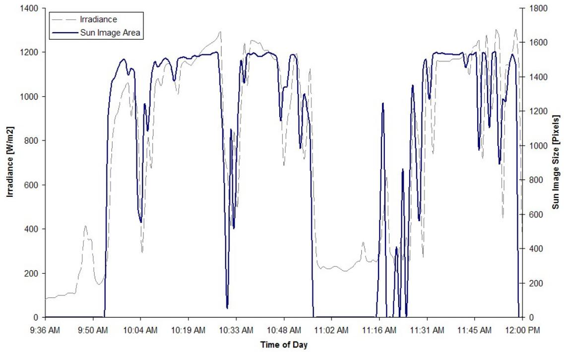
Fig. 8. Correlation of sun image size with independently measured global irradiance.
