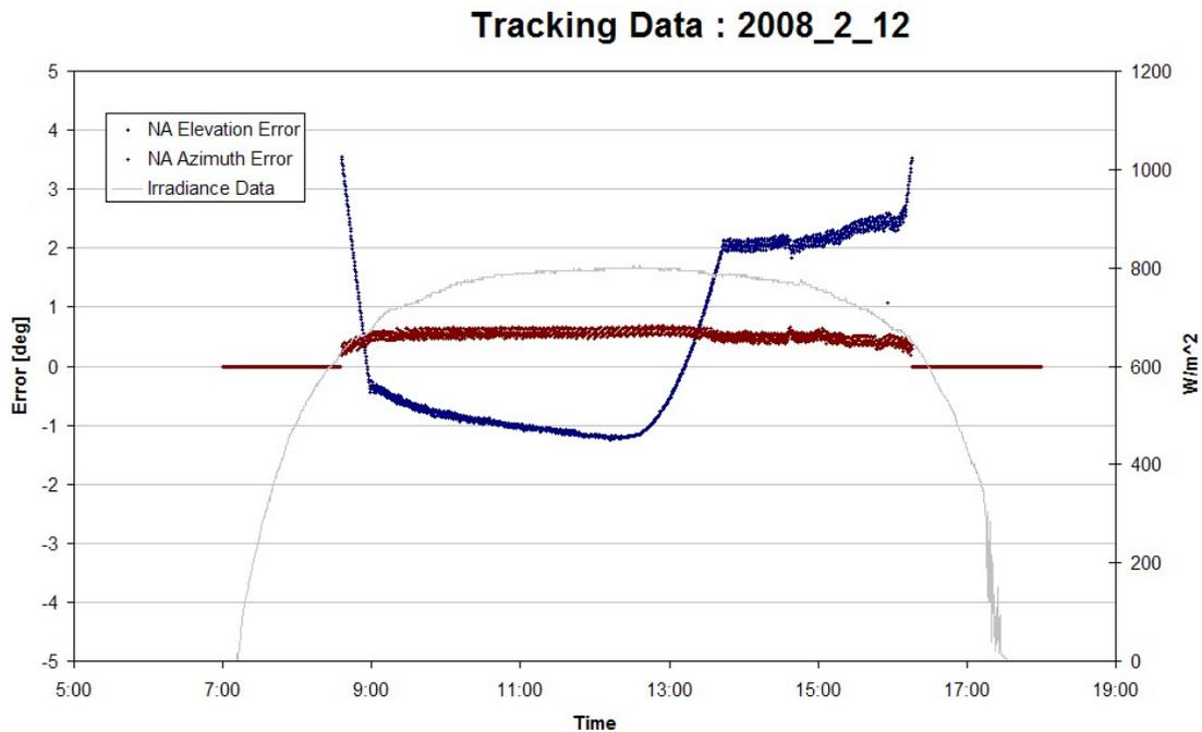
Fig. 5. Tracker performance as measured on a clear day.
