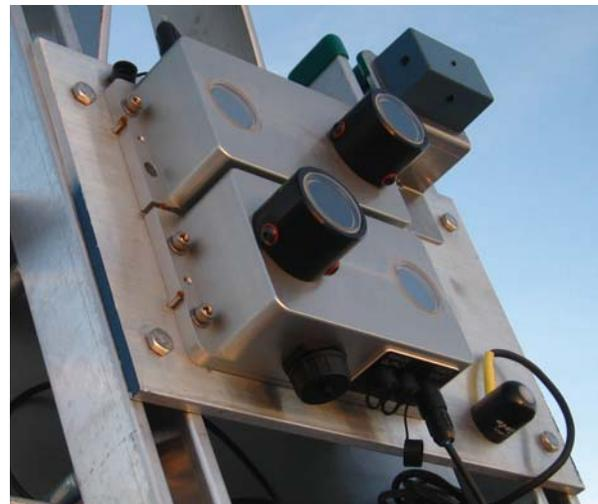
Fig. 1. Two Trac-Stat SL1's being tested in parallel.
